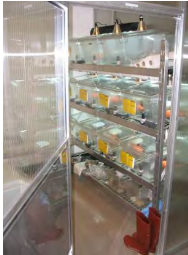
Figure 9. Lighting accommodated into the racks.
